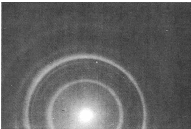
FIGURE 8 Electron diffraction pattern of the as prepared Na(acac).
